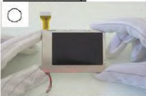
As above picture, please handle with anti-static gloves around LCM edges.
