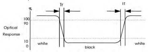
FIG 3. Measuring method for contrast ratio, surface luminance, Luminance uniformity, CIE (x,y) chromaticity.
