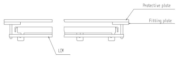
1.1.2 When assembling the LCM into other equipment, the spacer to the bit between the LCM and the fitting plate should have enough height to avoid causing stress to the module surface, refer to the individual specifications for measurements. The measurement tolerance should be  $\pm 0.1$ mm.
