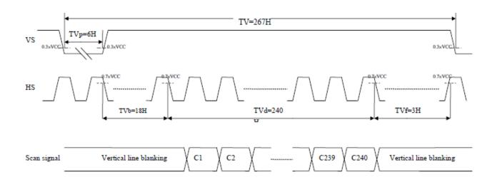
8.2 SYNC mode timing (DE connect to GND)
