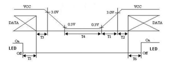
Timing Specifications: 0<T1≤15mS T2>0.5S 0<T3≤0.1S T4>1S T5>0.1S T6>0.1S
