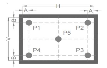
A:5mm /B: 5mm/H,V: active area/Light spot size= $\Phi$  5mm 500mm distance from LCD surface to detector lens of the BM-7
