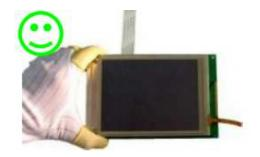
As above picture, please handle with anti-static gloves around LCM edges. 像上面的图片,请戴抗静电手套,并拿模块边缘.
