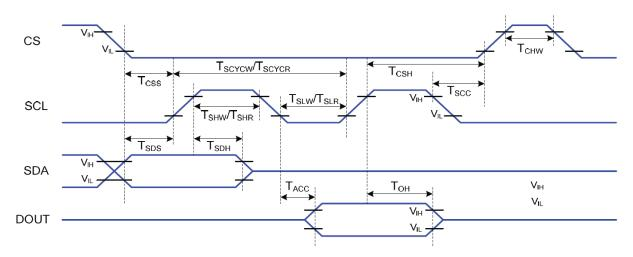
Figure 6-2-1 3-line serial Interface Timing Characteristics
