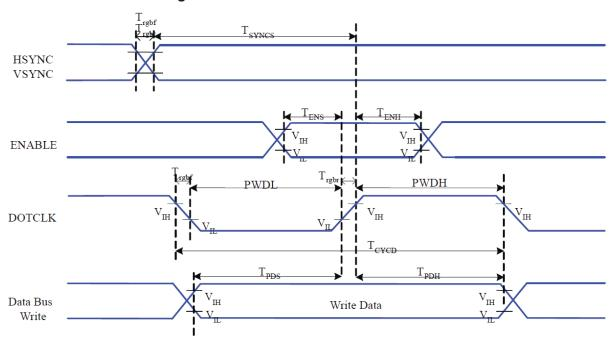
Figure 6-4-1 RGB Interface Timing Characteristics
