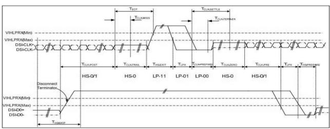
Clock lanes-High Speed Mode to/from Low Power Mode Timing
