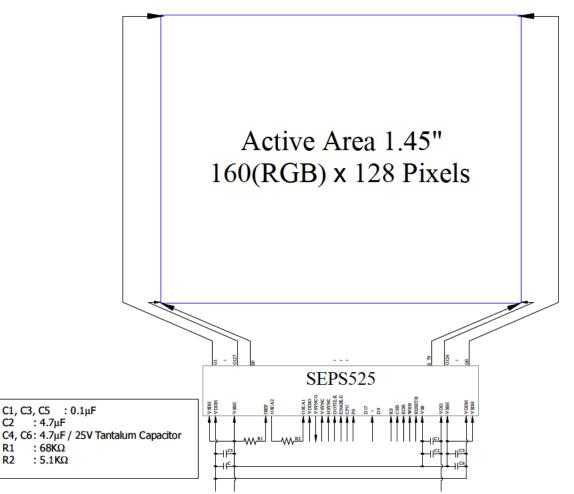
MCU Interface Selection : Base on CPU \ PS connection and Register setting (14h &16h). Pins connected to MCU interface : D17~D9, RS, CSB, RDB, WRB, and RESETB. Pins connected to RGB interface : D17~D12, VSYNC, HSYNC, DOTCLK, and ENABLE.
