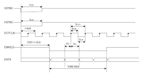
DTST: Setup Time for Data Transmission
