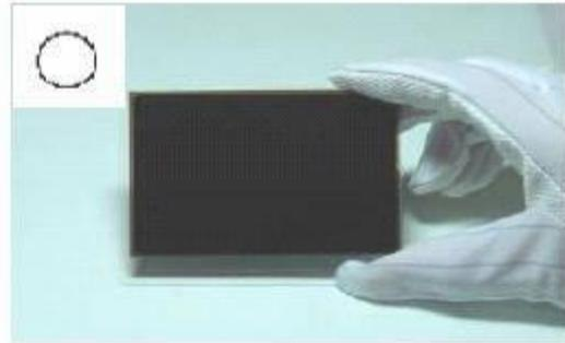
As above photo, please handle with anti-static gloves around LCD edges.
