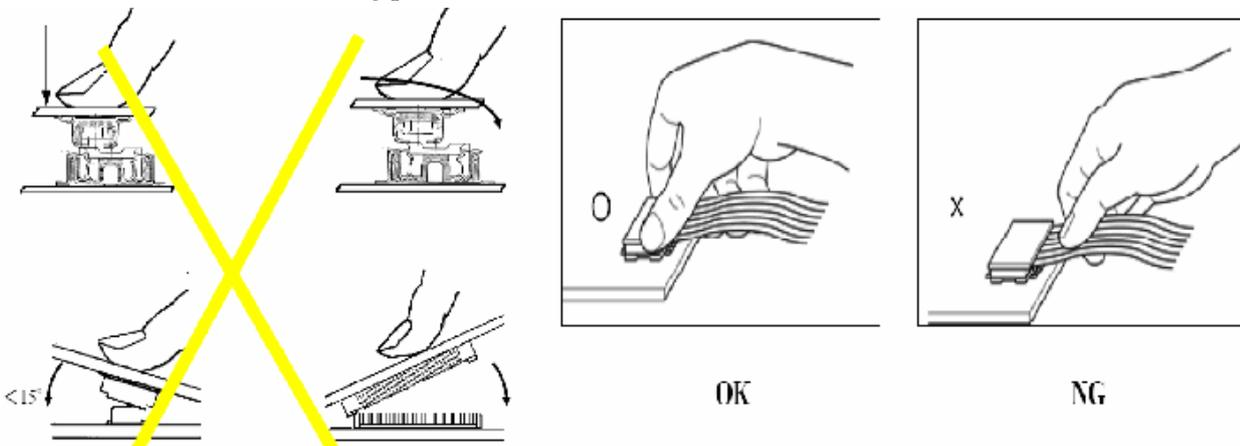
**Precaution for soldering to the LCM**
