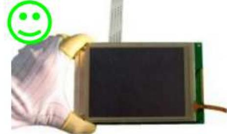
As above picture, please handle with anti-static gloves around LCM edges.
