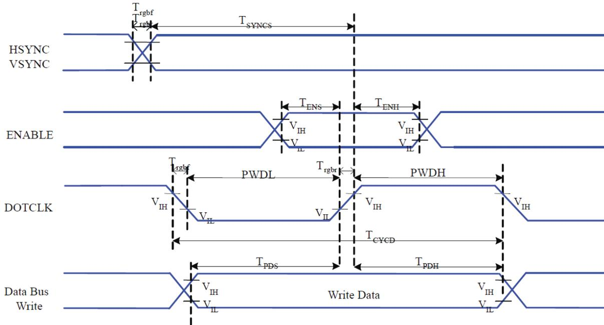
Figure6-4-1 RGB Interface Timing Characteristics
