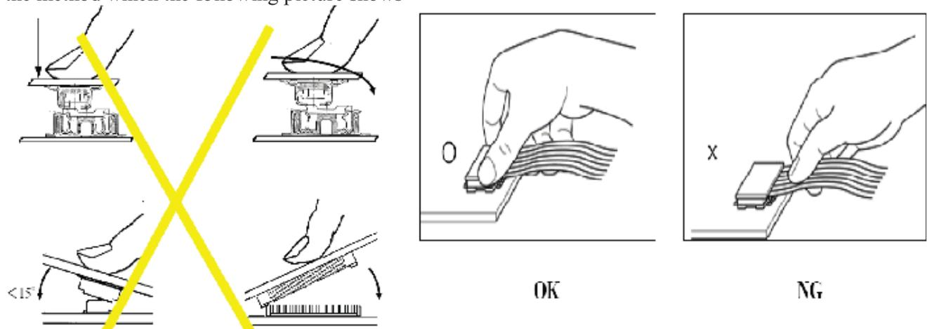
**Precaution for soldering to the LCM**
